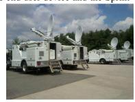
The Sprint SatCOLT is designed to be self-sustained over an approximate 5 day period based on actual usage and environmental conditions. In order to provide sustainable services over a period of more than 72 hours, Sprint employs a nationwide network of portable generators and multiple, national re-fueling contracts.
