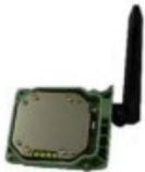
**Article** 798497 **Description** CGR4 UHF RTK radio expansion pack, 403-470 MHz radio Expansion Pack for all CS20 3.75G field controller variants. RTK receive only UHF radio to be easily attached to the CS20 expansion pack compartment. GAT26 RTK radio antenna not included.
