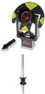
**Article** 641662 **Description** Mini prism GMP101, incl. bubble, target plate and spike, in bag, also suitable for GLS11 and GRT44 (same height as GPH1, additive constant +17.5mm)
