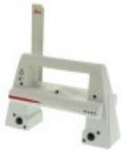
818467 RadioHandle with integrated long range Bluetooth module and radio antenna. Used as radio modem for Leica Viva TPS and Leica Nova instruments. Establishes communication to CS15 field controller or external radio modem TCPS29/30 (frequency range 2402 - 2480MHz, fulfils EN 300 328 V.1.8.1).
