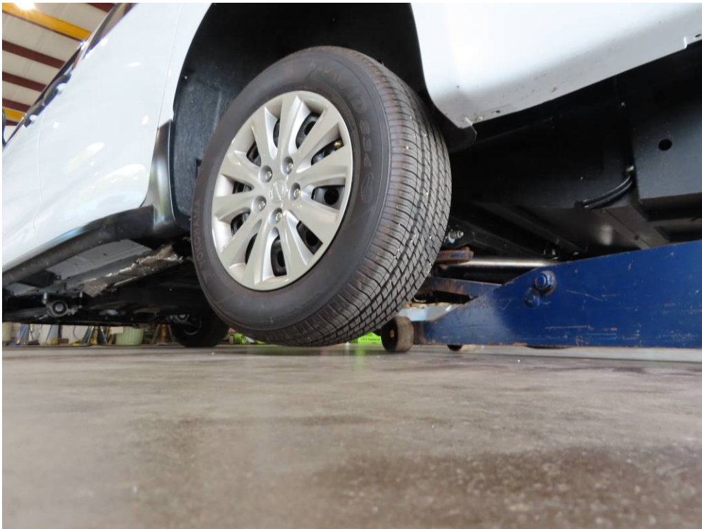
JACK IN PLACE – REAR
