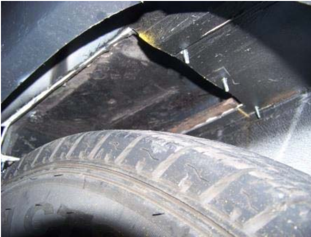
WHEEL WELL CUT OUT AND RAISED. (215 TEST MILES)
