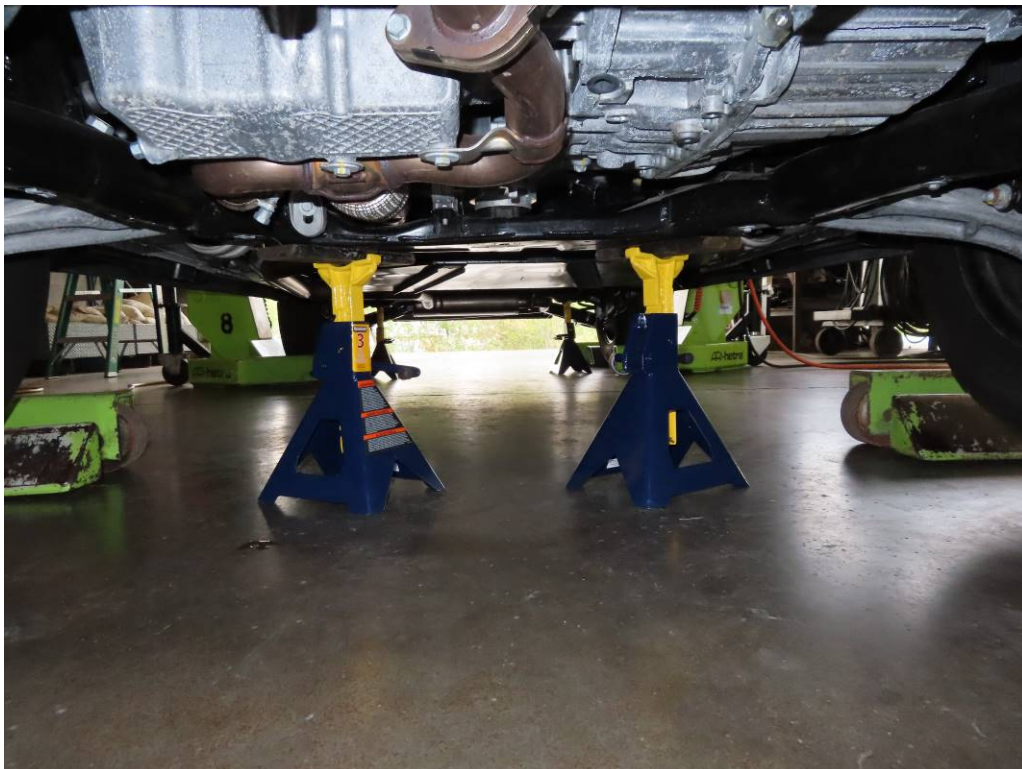
JACK STANDS IN PLACE – FRONT AND REAR
