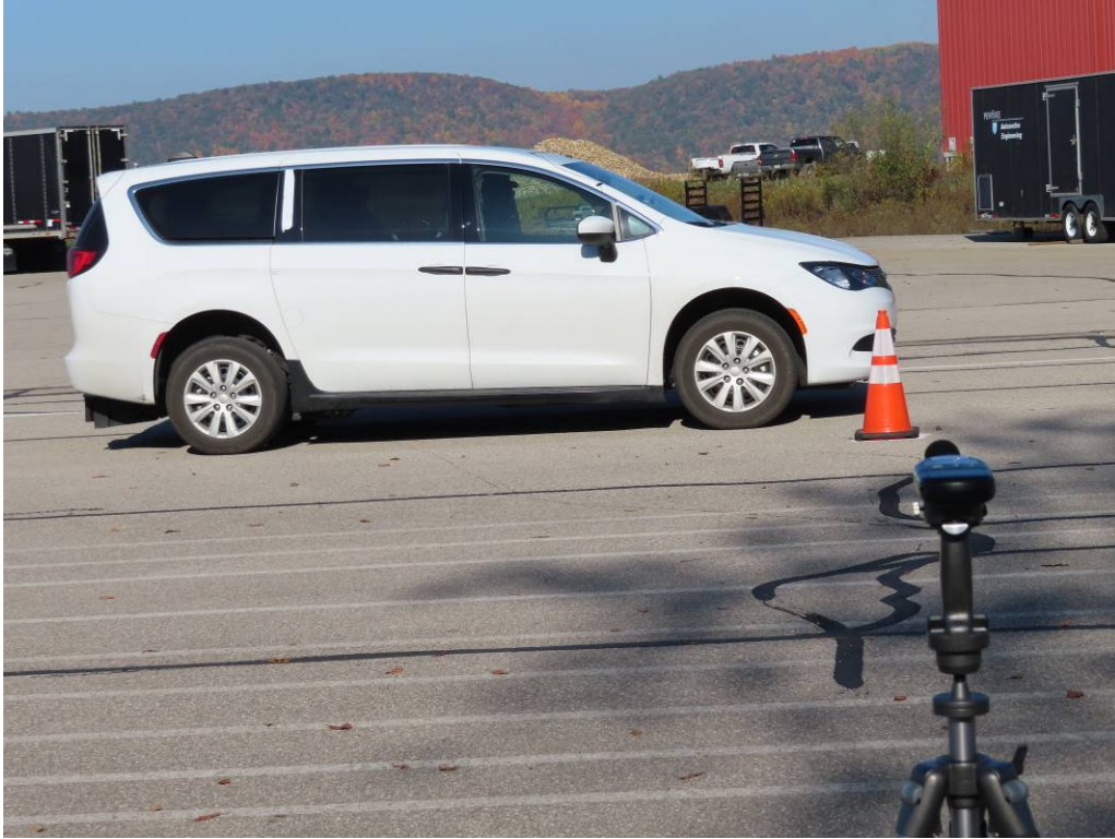
TEST BUS UNDERGOING EXTERIOR NOISE TESTING
