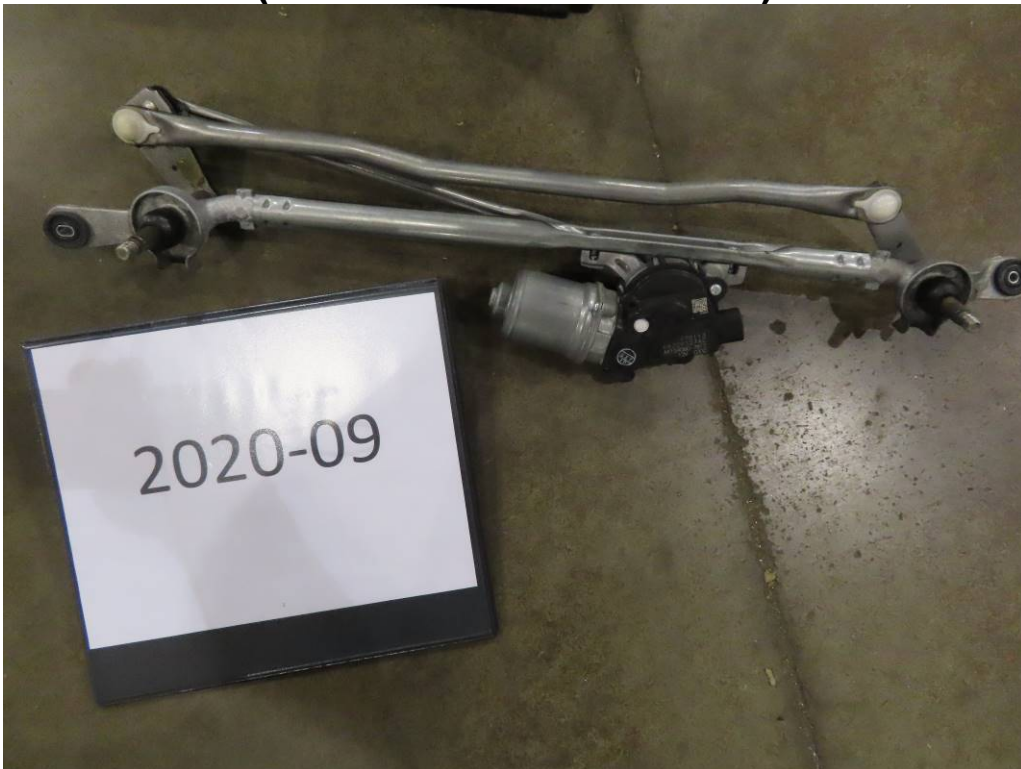
WIPER MOTOR REMOVAL AND REPLACEMENT (1.00 LABOR HOURS)
