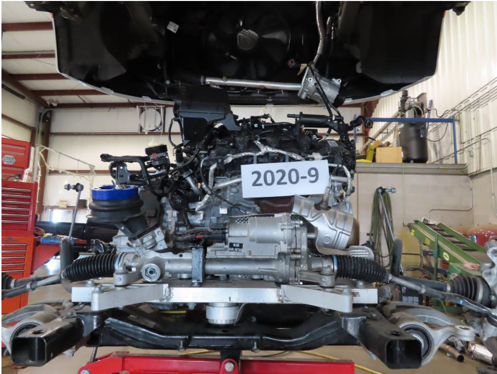
ENGINE / TRANSAXLE REMOVAL AND REPLACEMENT (10.00 LABOR HOURS)
