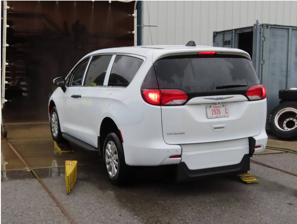
LEFT REAR WHEEL SIX INCHES LOWER
