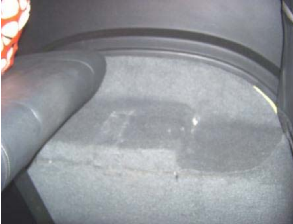
REAR WHEELS CONTACTING WHEEL WELL (215 TEST MILES)
