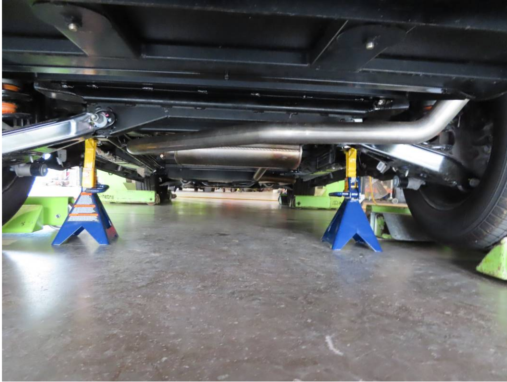
JACK STANDS IN PLACE – REAR
